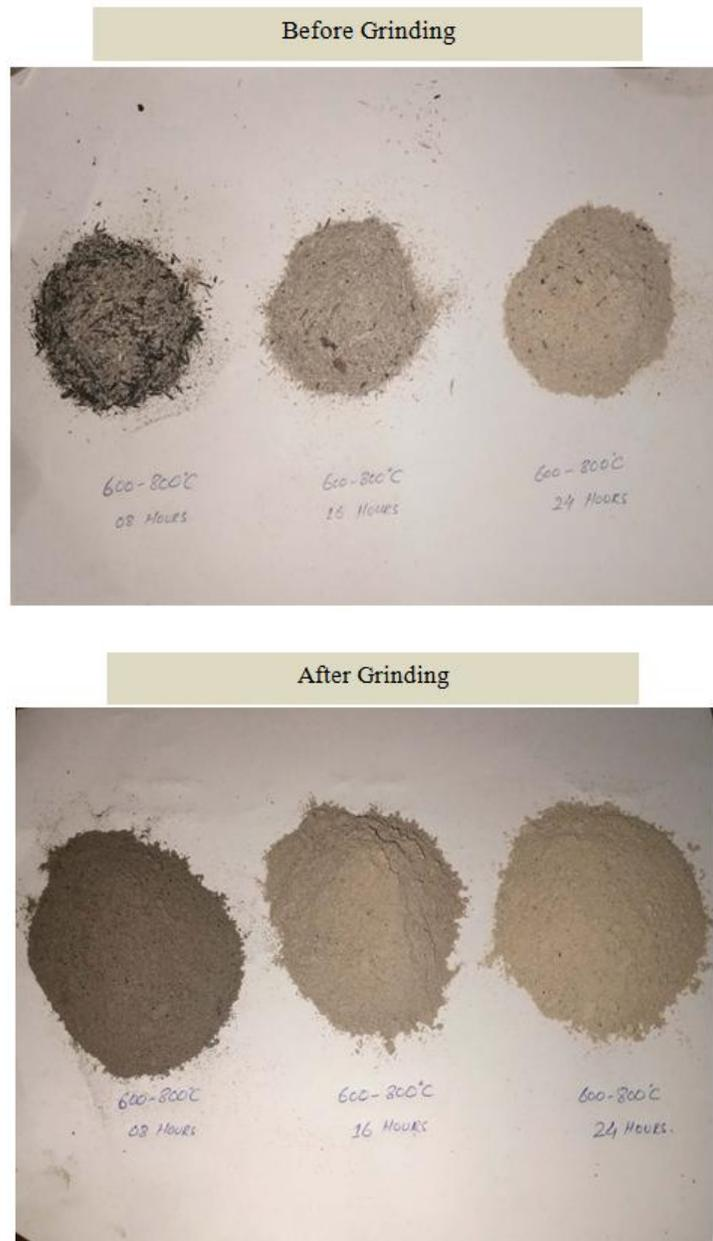
Fig. 2. Rice Husk Ash before and after grinding in ball mill
