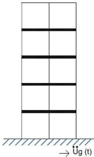
**Fig. 3(a). A multi-degree of freedom system subjected to ground motion**
