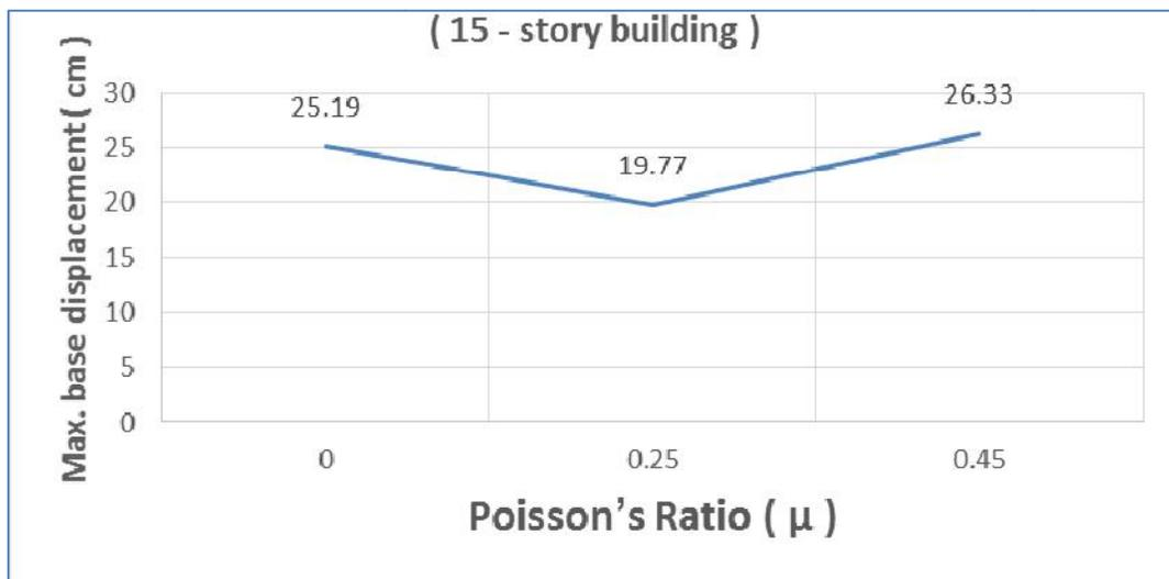
**Fig. 10. Relation between poissons ratio value and the max. base displacement**
