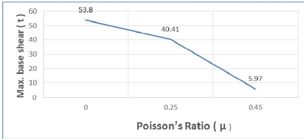
**Fig. 11. Relation between poissons ratio value and the max. base shear**
