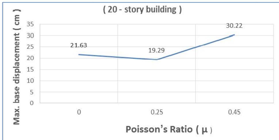
**Fig. 12. Relation between poissons ratio value and the max. base displacement**
