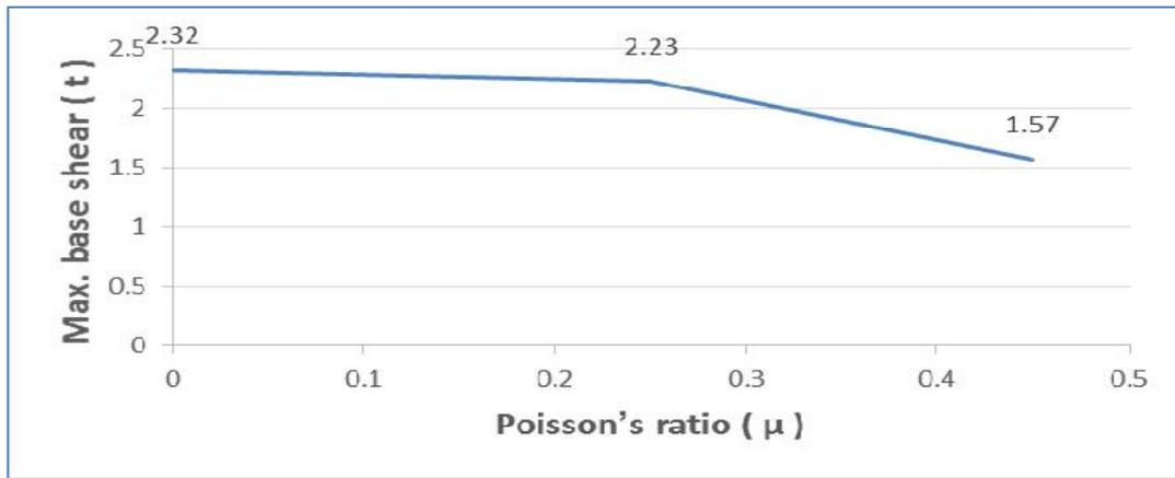
**Fig. 9. Relation between poissons ratio value and the max. base shear**
