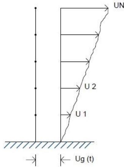
**Fig. 3(b). Lumped mass system and displacement**
