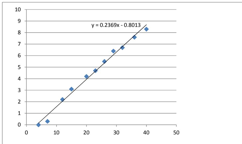
**Fig. 2. Calibration graph for the soil moisture content devise**
