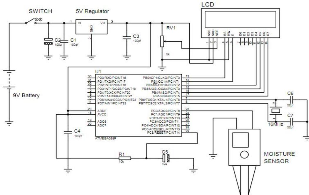
Fig. 1. Circuit diagram of soil moisture measuring devise
