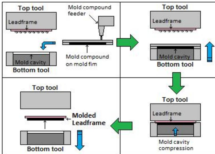
**Fig. 5. Compression molding mechanism**
