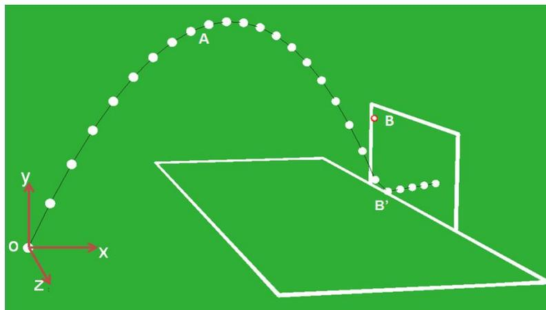
Fig. 3.6 A soccer ball shooting motion verse time 2.5 s with initial velocity  $v_0=12$  m/s, initial projectile angle  $\theta_0=60^\circ$ , and an initial orientation angle  $\beta_0=30^\circ$
