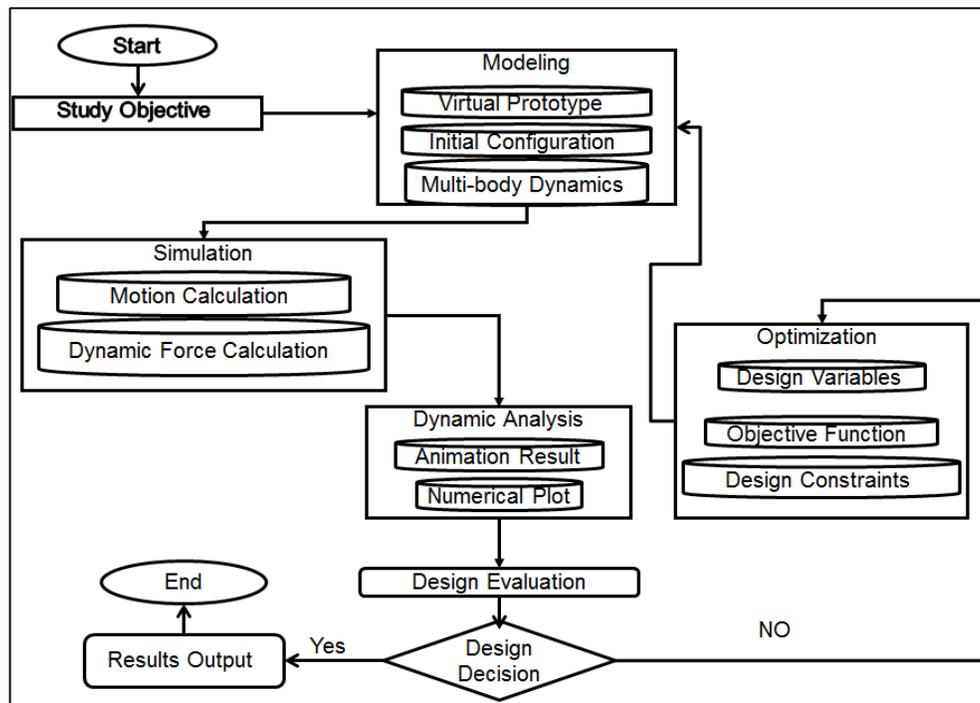
Fig. 2.3. A flow chart for modeling, simulation, and optimization of soccer ball shooting a target
