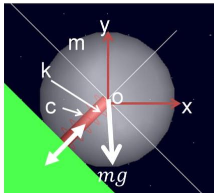
Fig. 3.5. A ball-body contact model with a mass-damping-stiffness system
