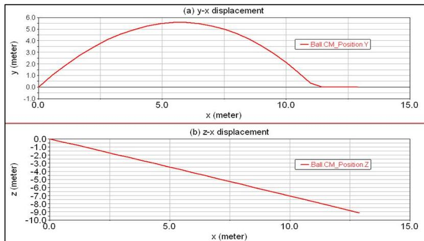
**Fig. 4.3. A soccer ball displacements verse time 2.5 s: (a) in x-y plane and (b) in x-z plane**
