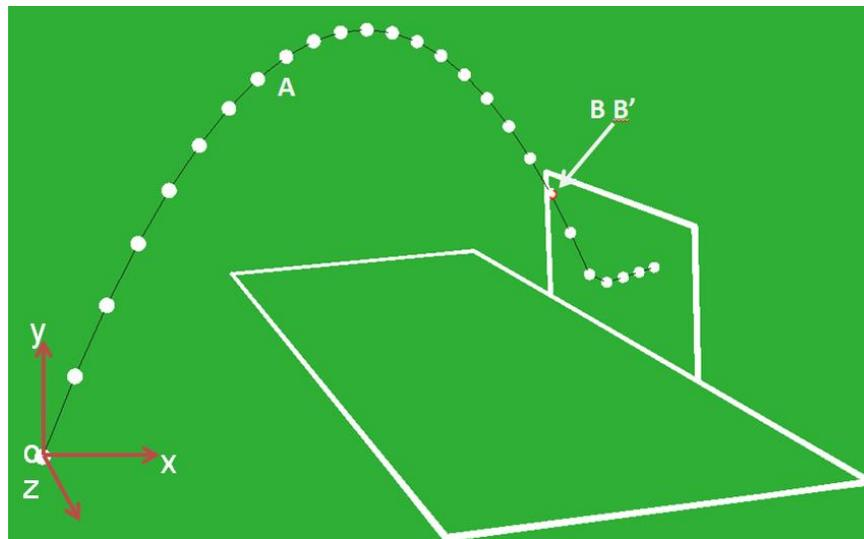
Fig. 4.2. A soccer ball shooting a goal with the initial velocity  $v_0=12.844$  m/s, initial projectile angle  $\theta_0=57.705^\circ$  and initial orientation angle  $\beta_0=34.575^\circ$
