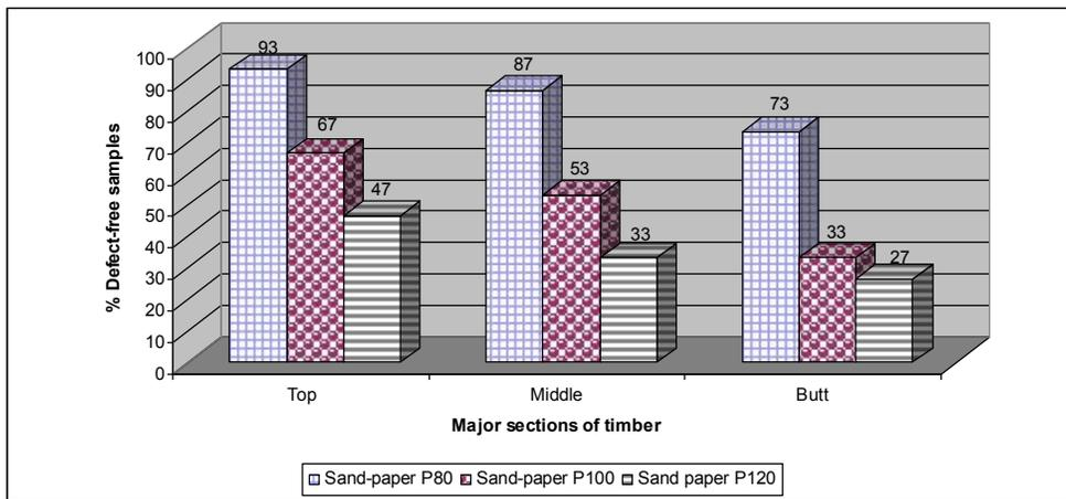
**Fig. 5.** Percentage of defect-free samples of sanded boards of three sections of *Gmelina arborea* trees from DSDFZ using P80, P100 and P120 sandpapers to eliminate chipped/torn grain defects
