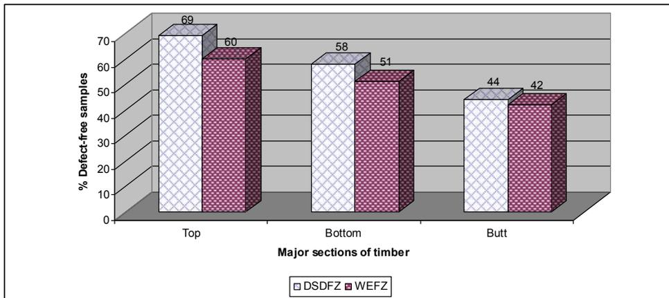
**Fig. 6.** Overall percentage of defect-free samples for sections of *Gmelina arborea* trees of two ecological zones using P80, P100 and P120 sand papers to eliminate chipped/torn grain defects
