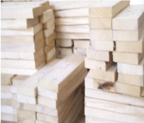
**Fig. 2. Specimens of *Gmelina arborea* wood prepared for shaping**
