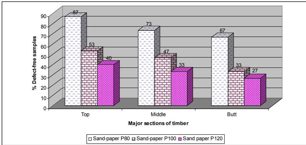
**Fig. 4. Percentage of defect-free samples of sanded boards of three sections of *Gmelina arborea* trees from WEFZ using P80, P100 and P120 sandpapers to eliminate chipped/torn grain defects**
