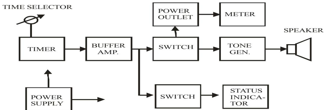
Fig. 1. Block diagram of the cooker control unit
