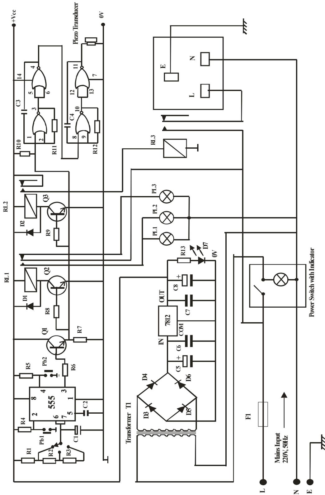
Fig. 8. Circuit diagram of the complete system
