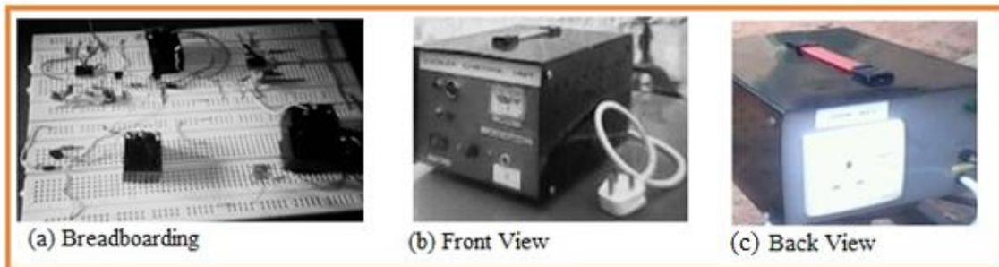
Fig. 7. The cooker control unit showing components wiring on breadboard and its completed front and back views
