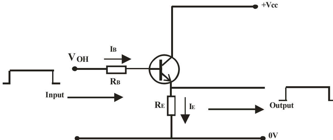
Fig. 3. A Common collector amplifier serving as a buffer
