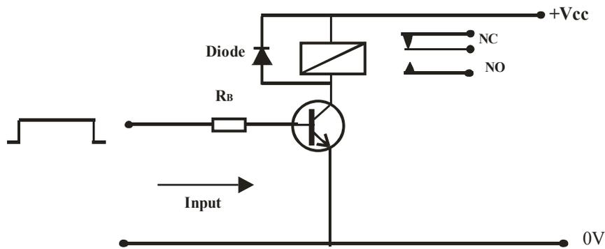
Fig. 4. Common emitter amplifier with a relay load
