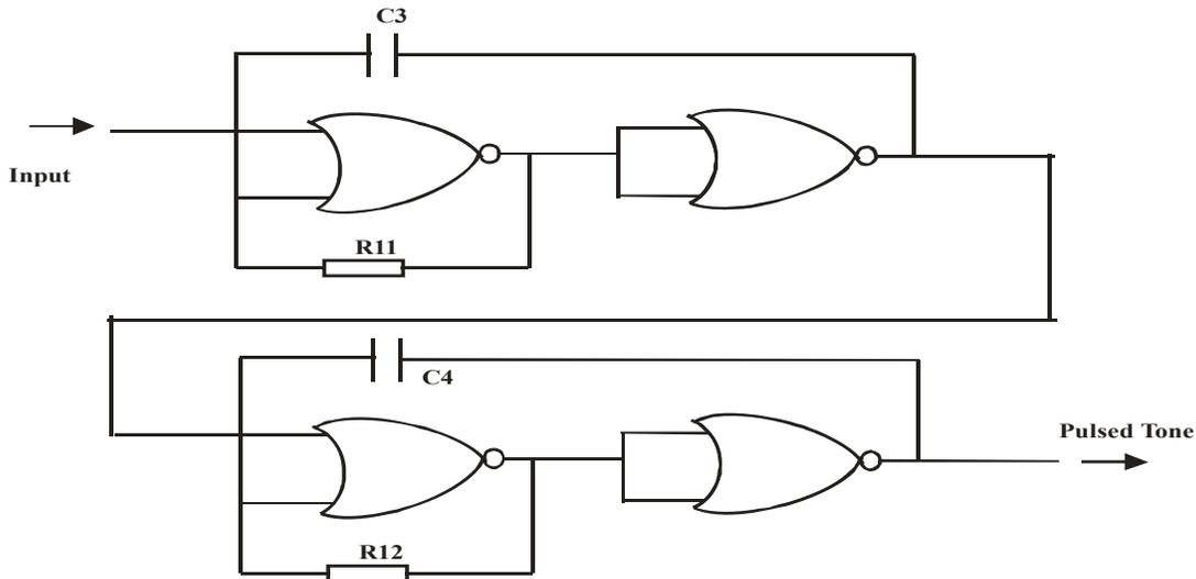
Fig. 5. NOR gates configuration
